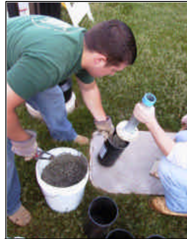
Figure 14 - Test Cylinder Preparation
